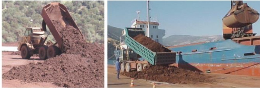
Figure 8: Left: Transportation and storage of Filtered bauxite residue as filter cake at storage site in Mytilineos, Right: Loading on a ship for use in a cement plant.
