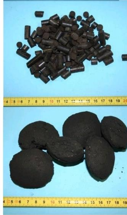
Char (at low volatile matters and low porosity) in pellets and briquettes for charging with basket
